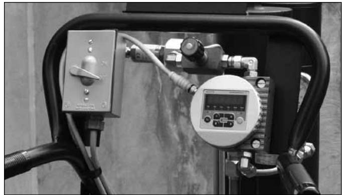
The CS1000 contamination sensor mounted on a filter cart.
